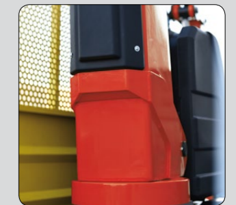
Robust column design and hoses cover
