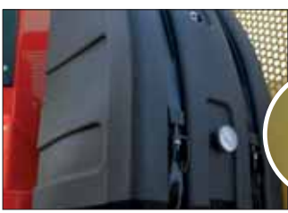
High volume oil tank made in sandwich-structured materials.
